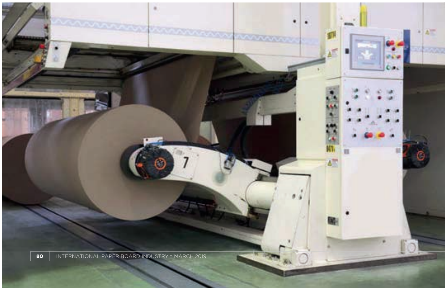
Turborex pneumatic roll stand brake installed in 2013.
